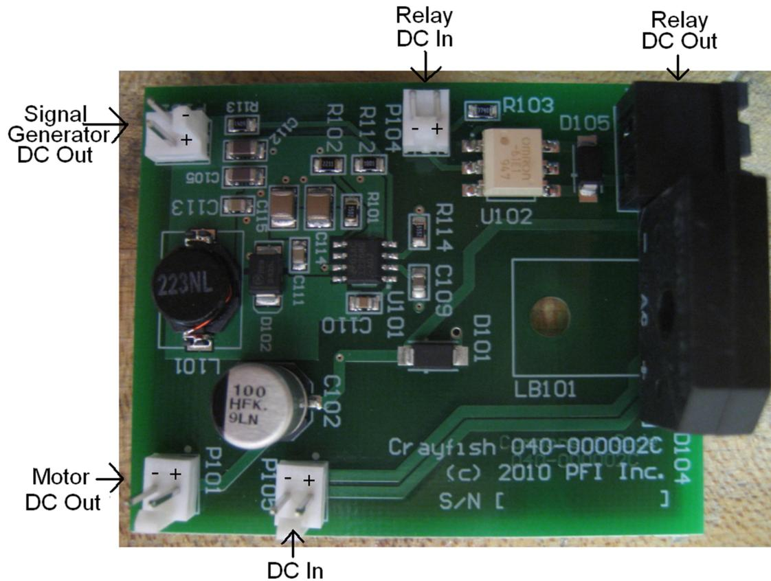
The function of the Power Board is to supply DC voltage to the drive modules as well as the logic signals to the Signal Generator. A schematic can be found in the Appendix
