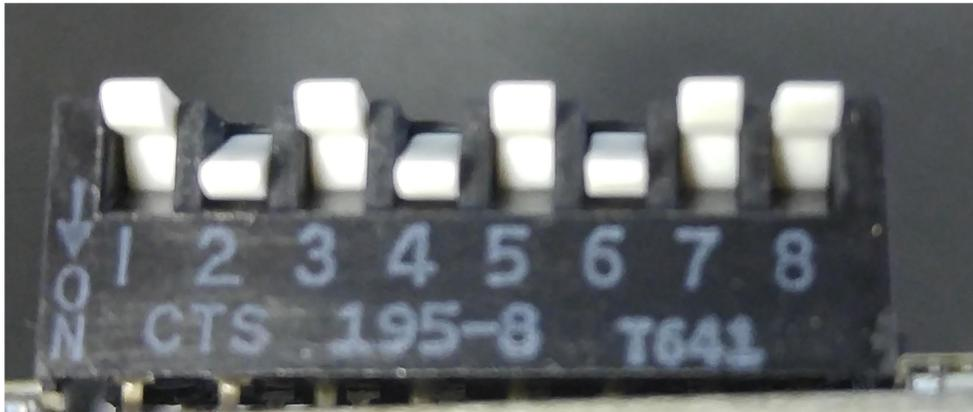
The switch is marked with the switch numbers and with an arrow showing which position the switch is **ON**.
