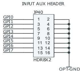
PINOUTS ARE FOR 1:1 MAPPING TO MINI-FIT JR.
