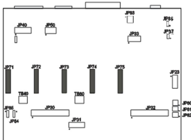
The Axis plug-in interfaces are used to add additional functions to the main signal generator board. For example, a stepper drive plug-in card or cable will enable you to drive a stepper motor directly from the signal generator box.
