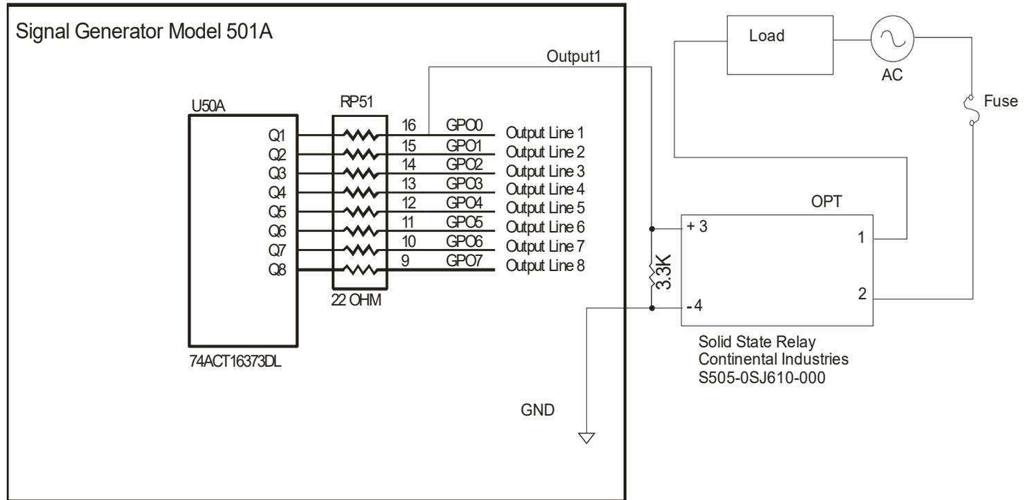
The above schematic shows a typical connection of one solid state relay controlled by output line 1 of the Signal Generator. A typical load would be a spindle, a vacuum, a laser, etc. In this example, the solid-state relay used is a Continental Industries model S505-0SJ610-000. It takes a 3 to 32VDC input and has an output of 24-330VAC.
