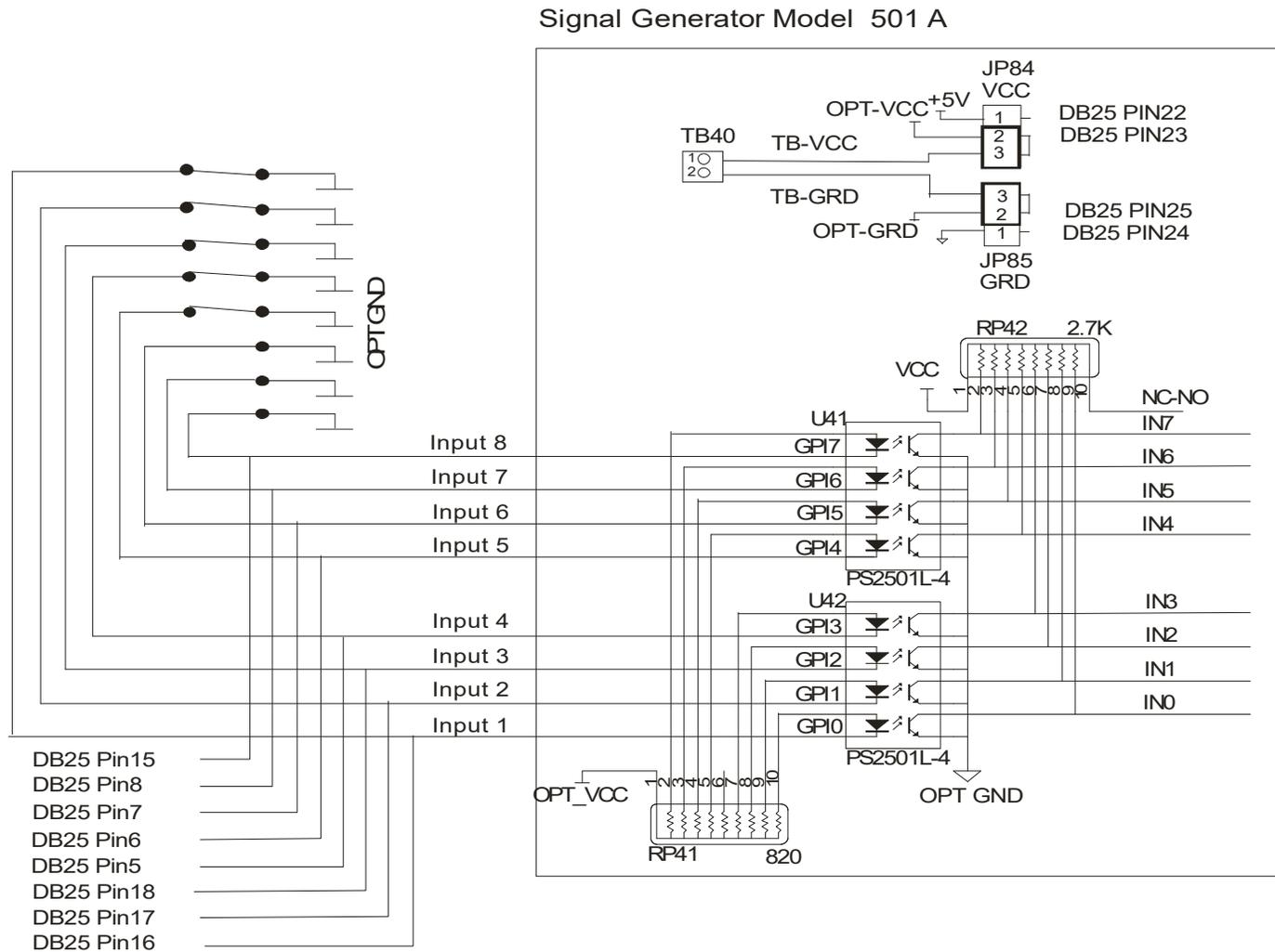
The above schematic shows a typical connection of 5 normally closed switches. These switches are connected between input lines 1-5 and ground. Lines 6-8 are connected directly to ground with jumper wires. All external connections shown are made through the Input connector on the back of the Signal Generator. This resistor pack (RP41) is socketed so that you can change the value if needed for your application.
