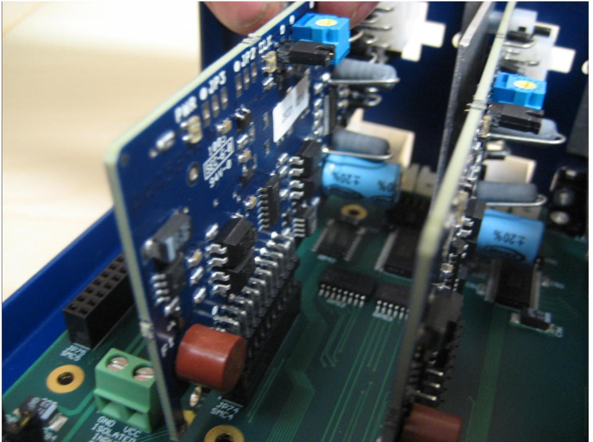
4. Mount the drive module to the driver box chassis using (1) #6 X ¼ self tapping screw.
