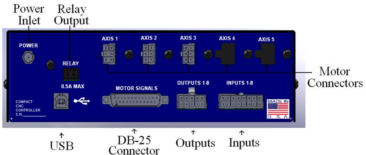
The rear panel has connectors for input and output signals as described below.
